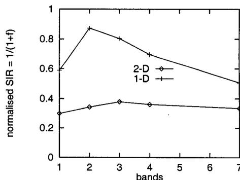
Fig. 5. Normalised SIR for different numbers of bands, in both one and two dimensional layouts.
