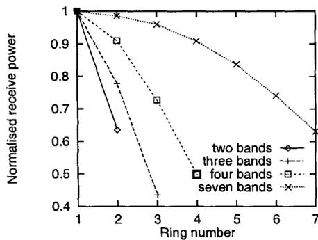
Fig. 6. Normalised received power for each ring , for 2, 3, 4 and 7 bands
