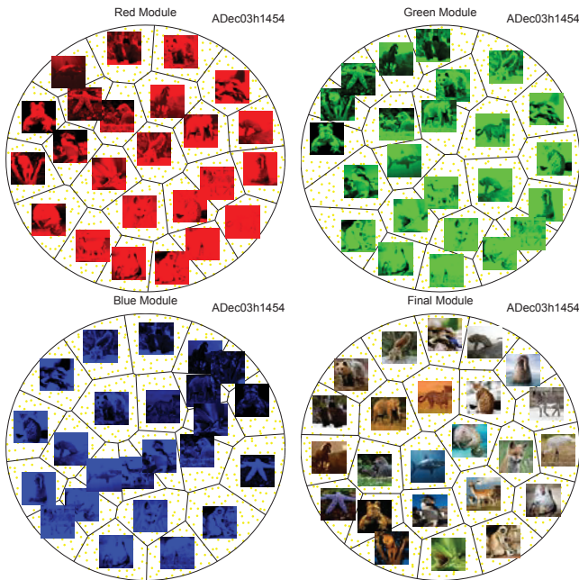
Fig. 4. Three first-level R, G, B maps and the final map representing categorization of colour visual object
