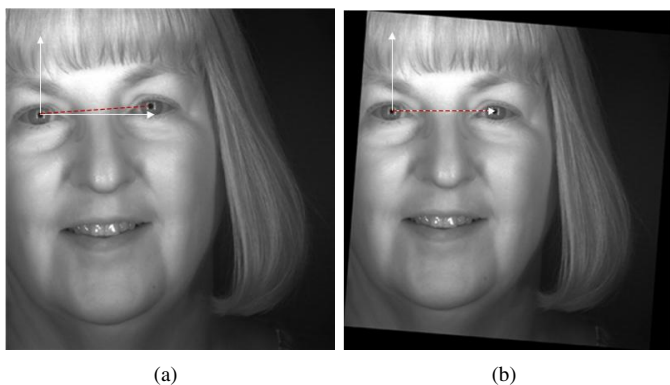
Fig. 4: Pupil Alignment: (a) is the reference frame, f_r (b) is the pupil aligned reference frame, f_a .
