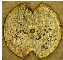
Figure 3. 1 mm diameter, 55 \mu\text{m} thick steel rotor used with the friction driven SAW motor. Notches were cut into each side to allow for visualisation of the high speed rotations.
