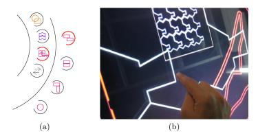
**Fig. 2.** (a) TILE main menu (Items listed top-down). Inner circle: region mode, Escher tiling mode, vector tiling mode, export/import. Outer circle (vector tiling mode selected): stretcher-bond, stack-bond, herringbone, packed circles. (b) A user manipulates an Escher tile pattern on the multi-touch panel.
