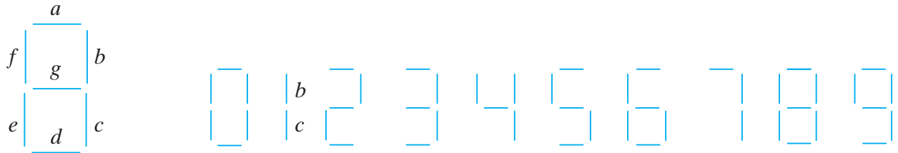
Figure 2: 7-segment display representation of decimal digits
