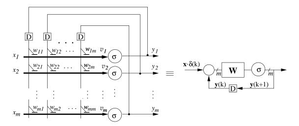
Figure 4: A dendritic and block diagram of a recurrent associative memory
