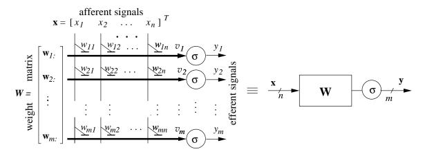
Figure 2: The structure of a feed-forward linear associator:  $y = \sigma(W \cdot x)$
