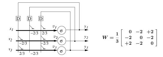
Figure 5: Example of a discrete Hopfield network with m=3 neurons: its structure and the weight matrix
