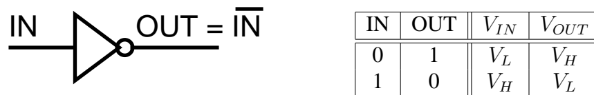
Figure 3.1: An inverter: logic symbol and the truth/operation table
