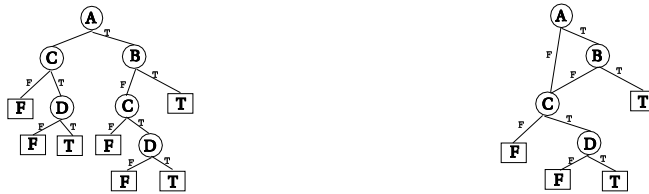
Fig. 1. Decision tree and Decision graph representations for (A \wedge B) \vee (C \wedge D)
