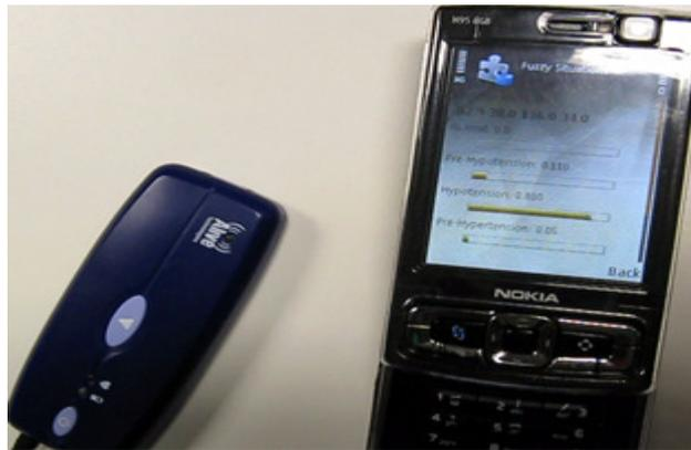
**Fig. 1.** The prototype of a FSI-based health monitoring application running on a Nokia N95 with an ECG biosensor
