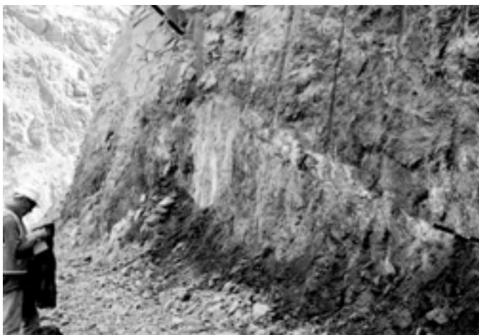
FIG. 12. Gently dipping, sheared contact between carbonaceous, pyritic Kapai Slate above and basalt below, at the North Orchin mine (Fig. 10).
