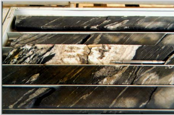
Fig. 2.5.17. Core from a high-grade intersection on the Centenary Line, showing a 30cm quartz vein within the strongly foliated Centenary Shale. Note the folded veins in the Shale, with axial-planes parallel to the foliation (width of view ~60cm).
