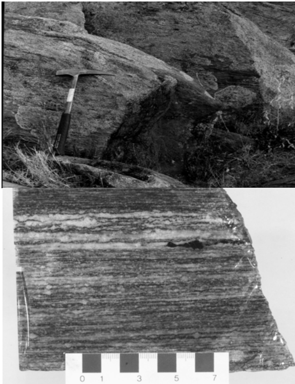
Fig. 2.5.6. a) Outcrop of Riverina Gneiss at Kurrajong highlighting the gently plunging mineral lineation. b) Polished slab of gneiss from the above locality, showing gneissic banding and lack of consistent asymmetries, indicating deformation was a product of essentially pure shear (scale bar in cm)
